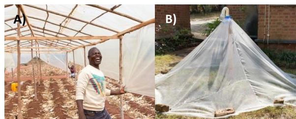
Figure 1 A) Inside a pilot rain-shelter built earlier this year to investigate design and logistics. B) Locally constructed emergence trap covering about 3 m 2 .
