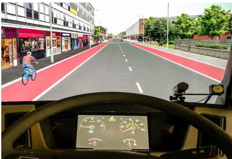
University of Leeds truck simulator is used for the design and testing of a system that informs drivers of potential collisions with cyclists in the XCYCLE project.
