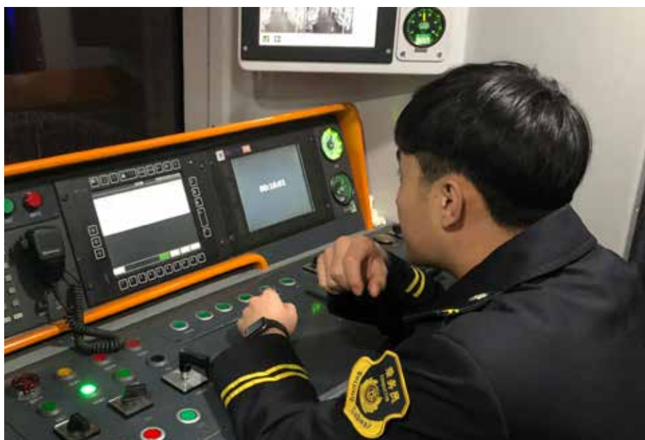
The ATO team successfully carried out a field trial on Line 7 of the Beijing Metro for energy-efficient automatic train speed control.
