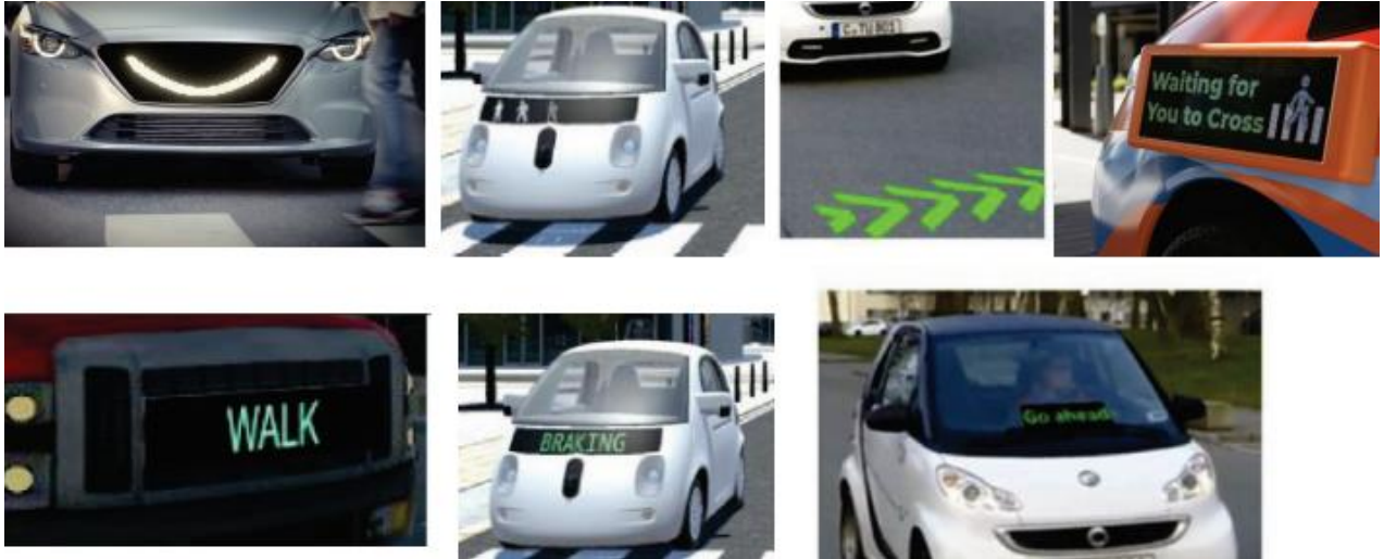
Some of the proposed external messages for interaction of automated vehicles with pedestrians. This is an extract from Prof Carsten’s Herman de Croo lecture.
