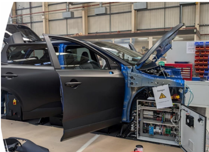
Computer systems are housed where the wheels in a standard car would be
