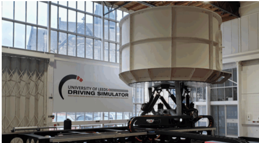
Refurbished housing for the Nissan Qashqai vehicle cab
